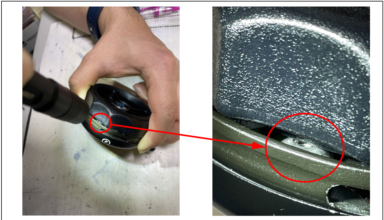
Figure 8 Side Belt Opening Inspection
