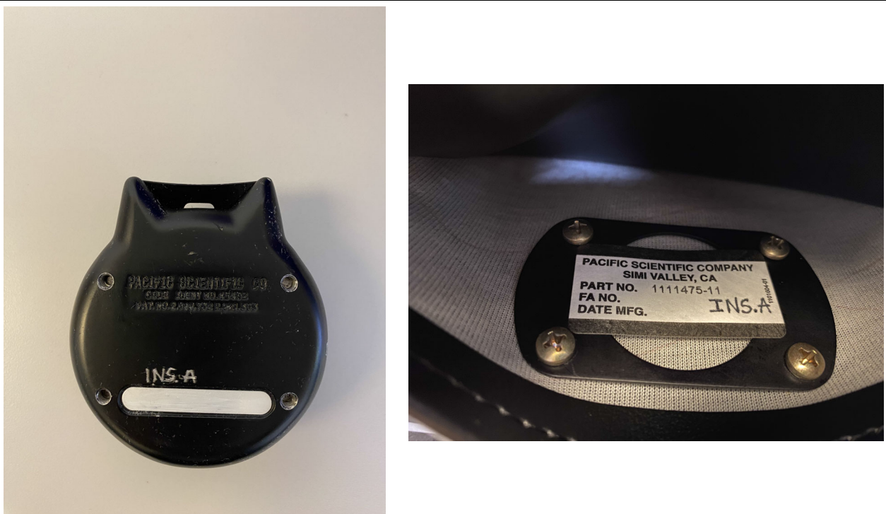
Figure 10 Re-Identified PNR 1111475 Series Rotary Buckle Assembly with "INS. A"
