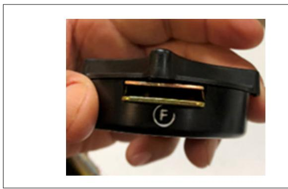
Figure 4 PNR 1111548-01 Rotary Buckle Openings for Inspection
