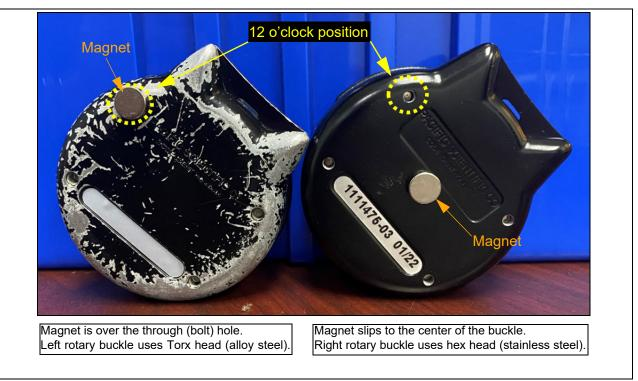
Figure 8 Magnet Test on PNR 1111475 Series Rotary Buckle
