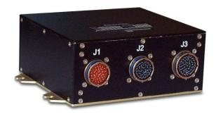
Our VCU-05 video control unit provides switching, power and control interface between aircraft systems and the camera system and/or security system. It incorporates a video switcher for direct selection of one of eight NTSC video sources and also passes all eight inputs through to the aircraft video distribution system.
