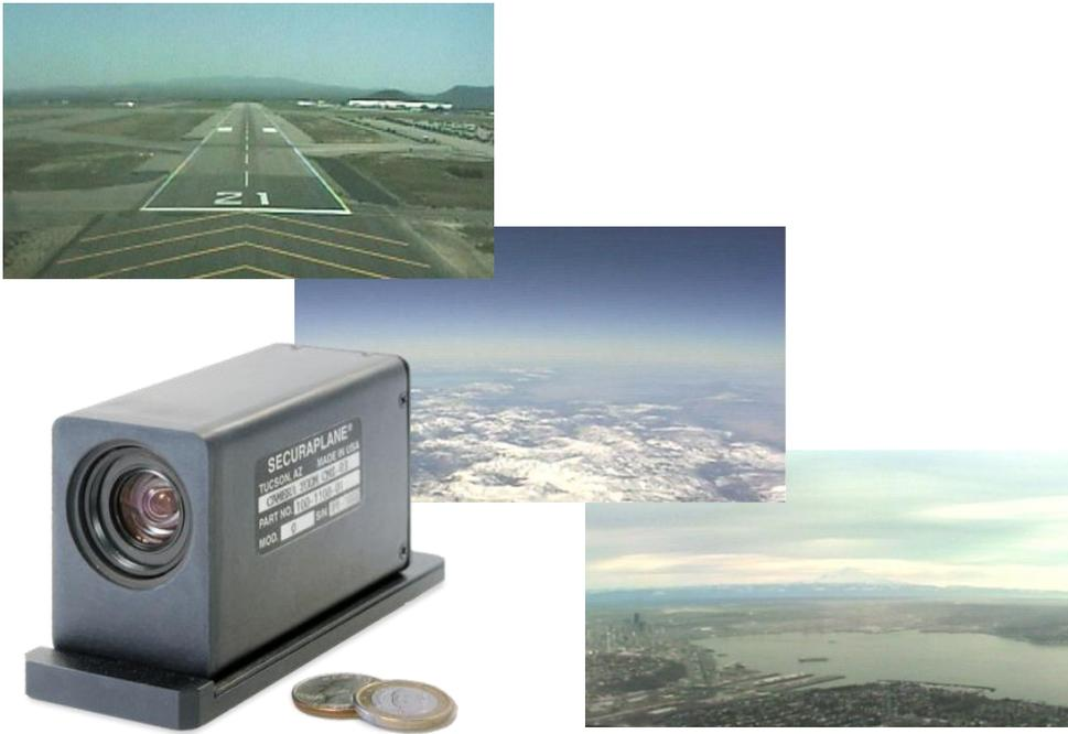
Securaplane's CMZ-03 Microzoom™ is a stand-alone glare shield color camera with a 40x telephoto zoom. This camera unit will operate directly from +28 VDC aircraft power and can be controlled via direct connection discrete keylines. The CMZ-03 also will operate on +12 VDC and offers digital bus control so it can interface to Securaplane's VCU-05 Video Control Unit for retrofit or system installations.
