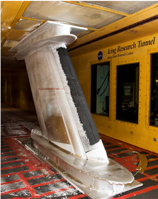
Electro-thermal Leading edge Wind Tunnel Test
