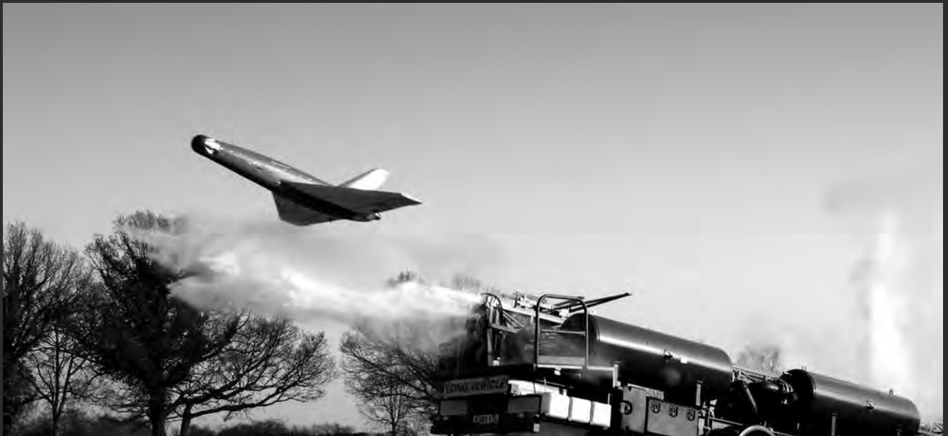
Herculean task: Meggitt Target Systems' 6,000 kg, 9 x 2 metre Hercules pneumatic catapult is designed to launch an aerial target weighing up to 250 kg at speeds of up to 55 metres per second with a launch pressure of between 2.5 to 10 bar.
