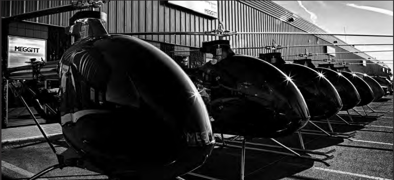
The new Mosquito pilotless helicopter target should enter full-rate production by the end of 2015. It sharpens troops' reactions during training by undertaking pop-up manoeuvres, replicating the sudden appearance of enemy helicopters at short ranges and the emerging UAV helicopter threat. Early models are in service in the US and Canada.
