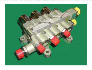
This valve manifold contains three solenoid valves, which direct pneumatic signals to the associated bleed valves.
